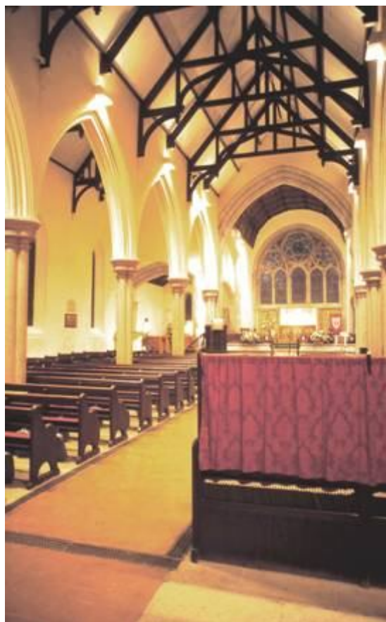
Figure 6. Holy Trinity Church in Salcombe using de luxe high pressure sodium lamps with their warm and welcoming colour rendering properties.
